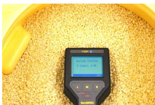
Fig. 6: Isotope identification test with fertiliser.
