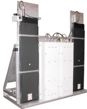
Detector side of skid
